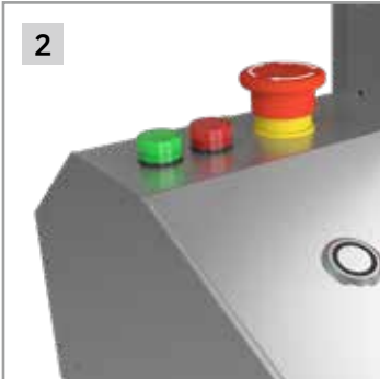
When you connect the power plug, the red light turns on.
