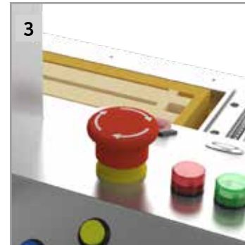
Turn the emergency switch clockwise (right) to release the emergency. (The following functions work only when the emergency is lifted)
