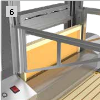
Hive controller loads and store the honeycomb on the hanger.
