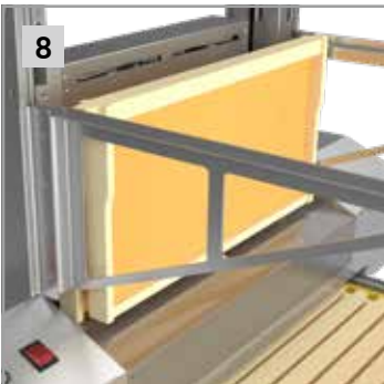
When the hive moves to the hive rack, the next hive is withdrawn.
