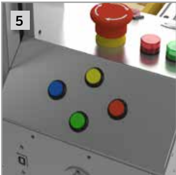
Press the button (up/down/front/back) of the operation unit to remove the jam/stick. (It does not work until the emergency switch is pressed for normal operation of the product.)
