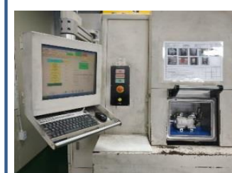
Helium Leak Test
