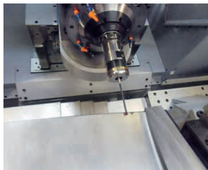
3D-measuring of a turbine blade in the HSTM
