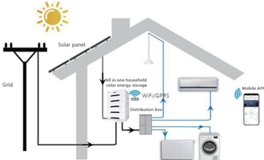
All in one solar energy storage is a multifunctional intelligent energy storage with inverter cabinet, integrating inverter, AC charger, photovoltaic charge controller and AC bypass. It has optional AC sources, an intelligent management system for AC chargers and solar charge controllers, and an energy management system for AC output, which guarantees customers' normal electricity consumption to the greatest extent and reduces the cost of customers' electricity consumption.
